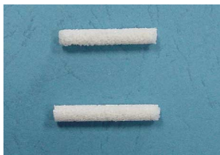
Fig. 5. Photographs of porous n-HA/PA66 scaffold materials.
